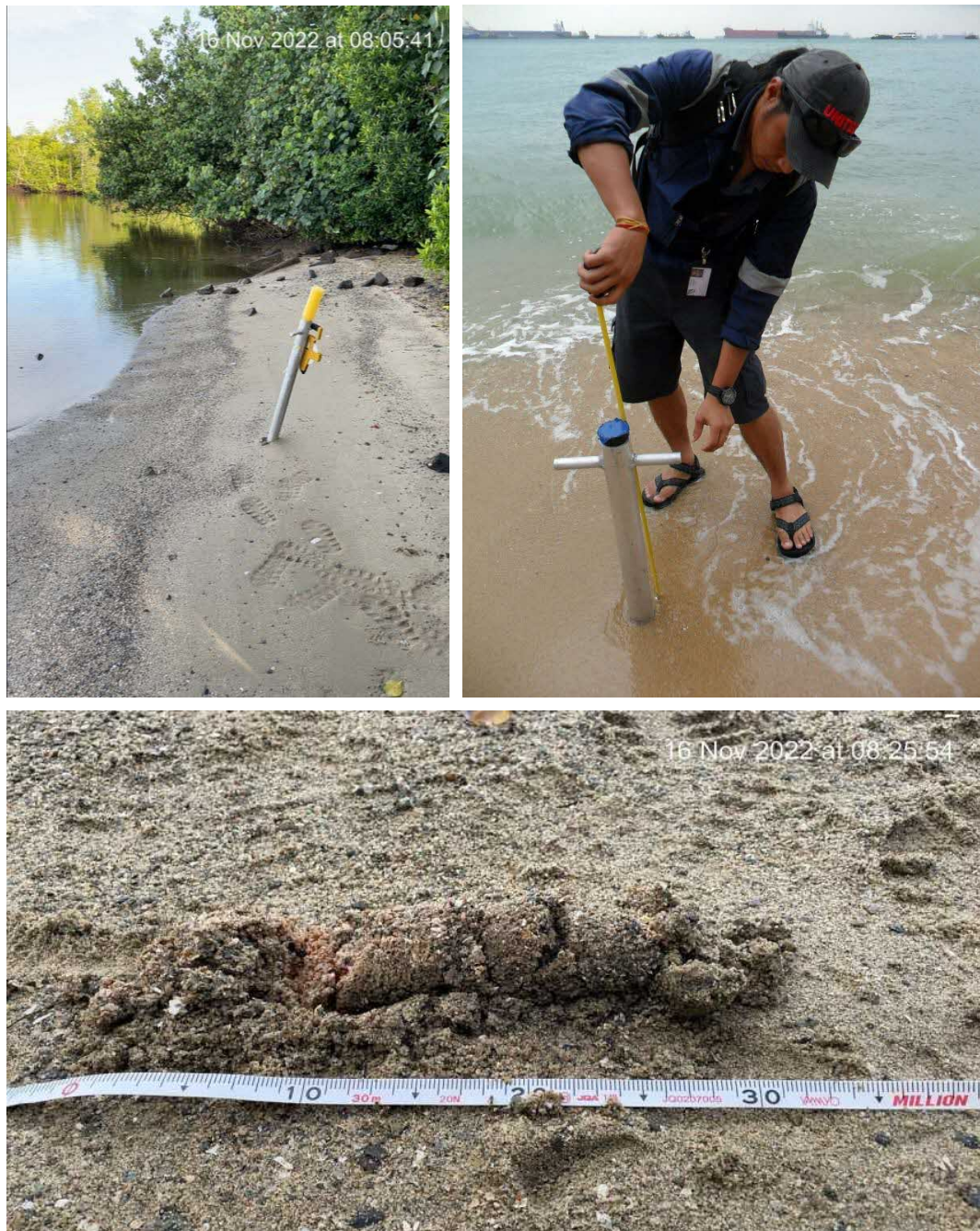
Figure 5.31. Hand auger sediment core location (top left), an example of the extraction process (top right), and final sample (bottom)
