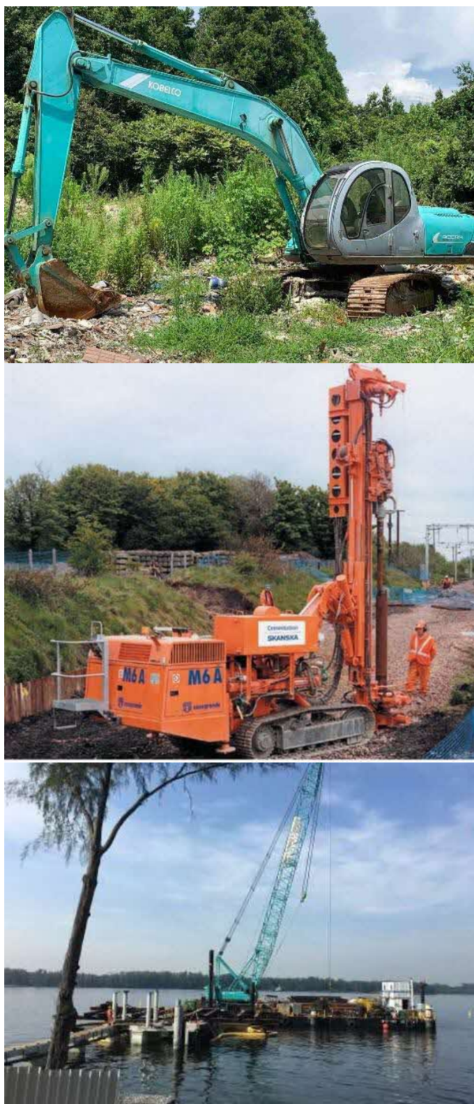
Figure 2.3 Construction equipment types to be used for the development (Top: for trimming of seabed; Middle: for micro piling; Bottom: for marine piling)
