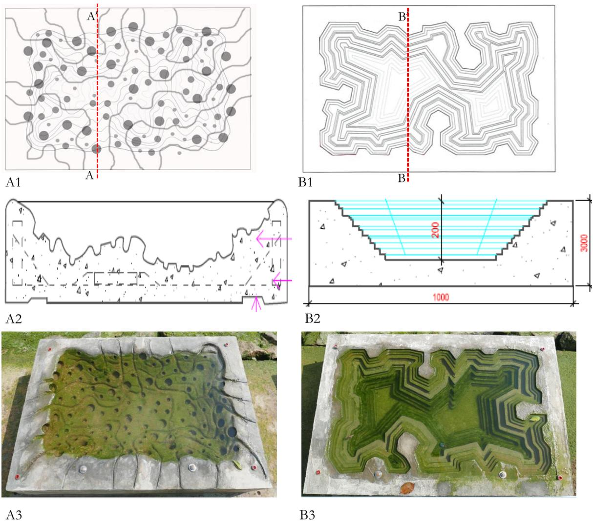
Figs. 2. (A) 1. Design of the pool with pits and grooves – Plan View; 2. Cross section A-A'; 3. Final cast of the pool with pits and grooves; (B) 1. Design of the pool with randomised steps – Plan View; 2. Cross section B-B'; 3. Final cast of the pool with randomised steps.
