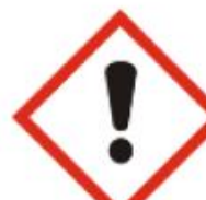
Acutely toxic(harmful), Irritant to skin, eyes or respiratory tract, Skin sensitizer, Hazardous to the Ozone layer.
