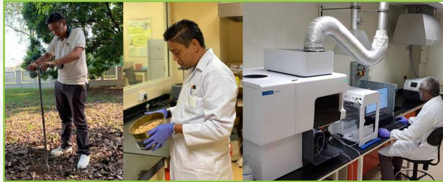
Conduct physical and chemical tests on soil, soil mixes and sand
