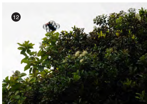
10. Inspections can be carried out within minutes even for areas of interest which are high up in the canopy, a process which would otherwise have taken hours to perform via climbing or crane.
