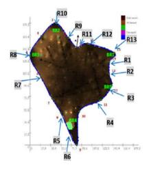
Tomogram results taken at lowest level at 150mm height indicates 99% sound and intact at the tested plane. Verification drills R1, R2, R4, R7, R9, R11 and R12 are carried out at a 45 degree angle at trunk base. R3, R5, R6, R8, R10 and R13 are carried out at buttresses.
