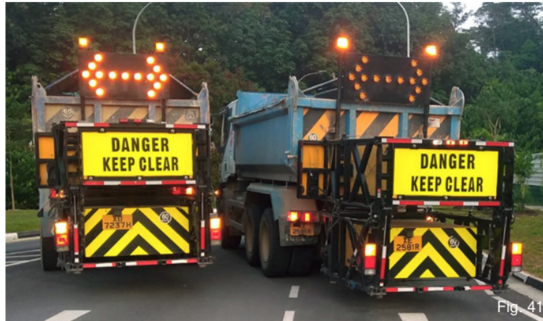
Truck Mounted Attenuator (TMA) - mount blinking beacon lights on the top and warning signs at the rear of vehicles
