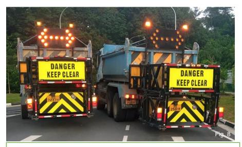
Truck Mounted Attenuator (TMA) - Mount blinking beacon lights on the top and warning signs on the rear of vehicles
