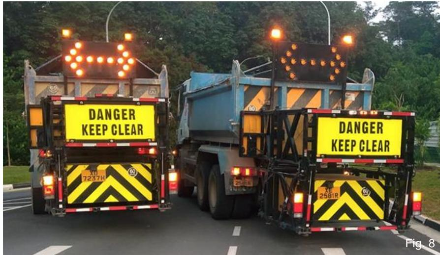
Truck Mounted Attenuator (TMA) - Mount blinking beacon lights on the top and warning signs on the rear of vehicles
