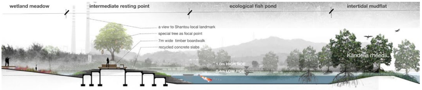
14 Typical cross section of the recreational fish pond.
