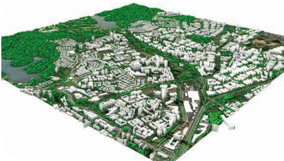
Fig 3. The figure shows the result of a research project looking to include trees in a digital twin of Singapore whereby 3D trees are parametrically generated using a combination of data sources from satellite imagery, GIS databases, and developed allometric equations (Lin et al., 2018).
