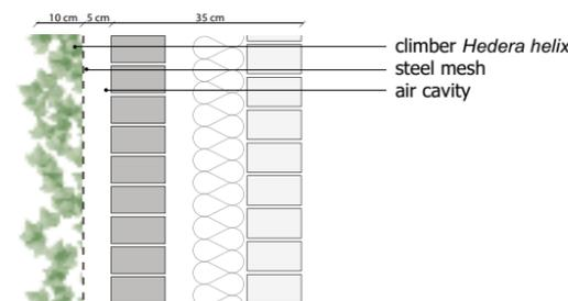
e. Indirect Façade Greenery Based on Stainless Steel Mesh
