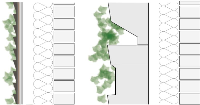
10. Illustration of higher integration into the building envelope in a living wall system-based concept. In this case, for a newly designed building, the traditional cladding system can be omitted. This results in a less expensive solution, faster building time, decrease of the environmental profile, and so forth.
