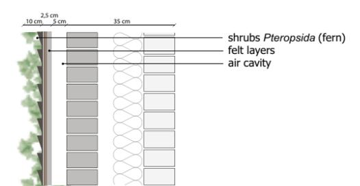
d. Living Wall System Based on Felt Layers
