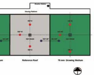
2. Schematic roof plan of the Research Facility showing the location of the green roofs (GR-1 and GR-2), instrumentation, weather poles (WP), and weather station
