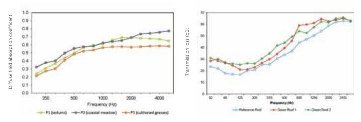
11. Measured absorption coefficients of three plant communities (in substrate depths of 125 to 200 mm) after two seasons of establishment
