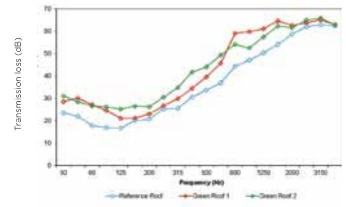
12. Measured transmission loss of three roofs at the Research Facility
