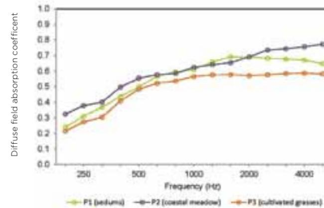
11. Measured absorption coefficients of three plant communities (in substrate depths of 125 to 200 mm) after two seasons of establishment
