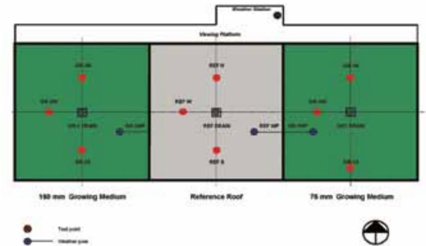
2. Schematic roof plan of the Research Facility showing the location of the green roofs (GR-1 and GR-2), instrumentation, weather poles (WP), and weather station
