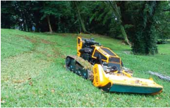
6. Robocut, a remote-controlled grass mower, is a safer and more efficient alternative to the more commonly used single-person ride-on mower (Photo: Chew Thiam Kwee).
