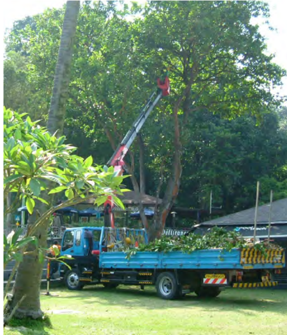
The ground must also be able to withstand the weight of the crane to carry out tree pruning
