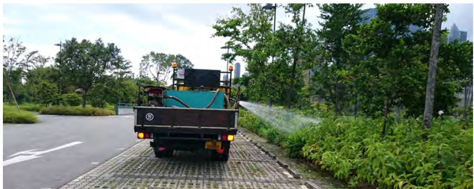
Automated tanker watering can be a one-man operation instead of deploying another worker to hold the hose sprinkler
