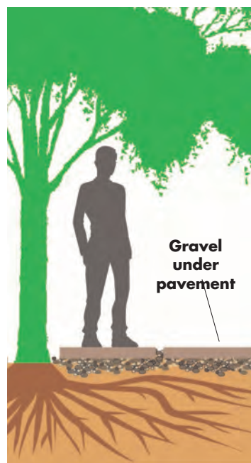
Gravel can improve aeration under footpaths
