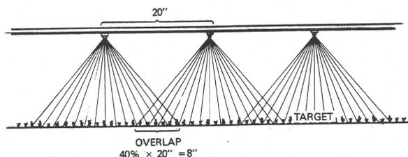
Fig 6. For uniform distribution, broadcast nozzles are designed for 40% overlap
