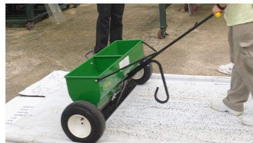
Fig 5. Calibrating a drop fertiliser spreader
