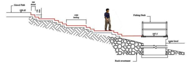
The same flight of steps could have been better designed with two landings inserted with adjustments to the threads:
