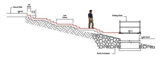
The multiple of 1500mm rule need not apply if the landing is more than 4500mm. This is because at this distance, user has sufficient time to adjust their strides comfortably before the next flight of steps. In such a case, it is more accurate to view this as a path with a series of steps built in rather then as a flight of steps with landing
