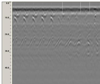
Left to Right: Fig 4. X-ray scan; Fig 5. Radar traces from a GPR scan
