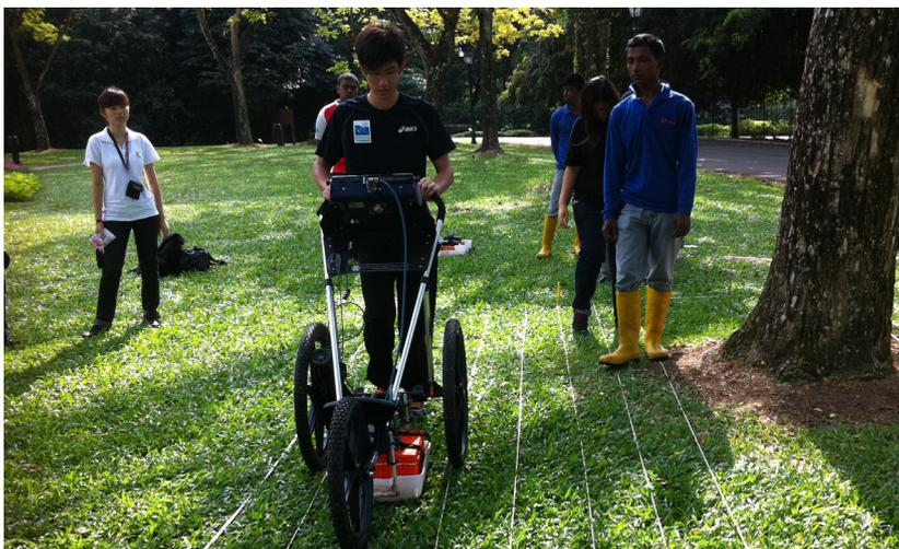
Fig 1. Tree root survey using the GPR
