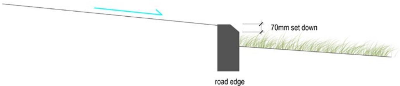
**Fig 4.** This photo shows leaf litter accumulating at water entry point where the grass is the same level as the road. To avoid this accumulation, a tapered flush kerb must be used that sets the top of the vegetation 70mm (as shown in the cross section), which requires the top of the ground surface (before turf is placed) to be approximately 100mm below the road surface.
