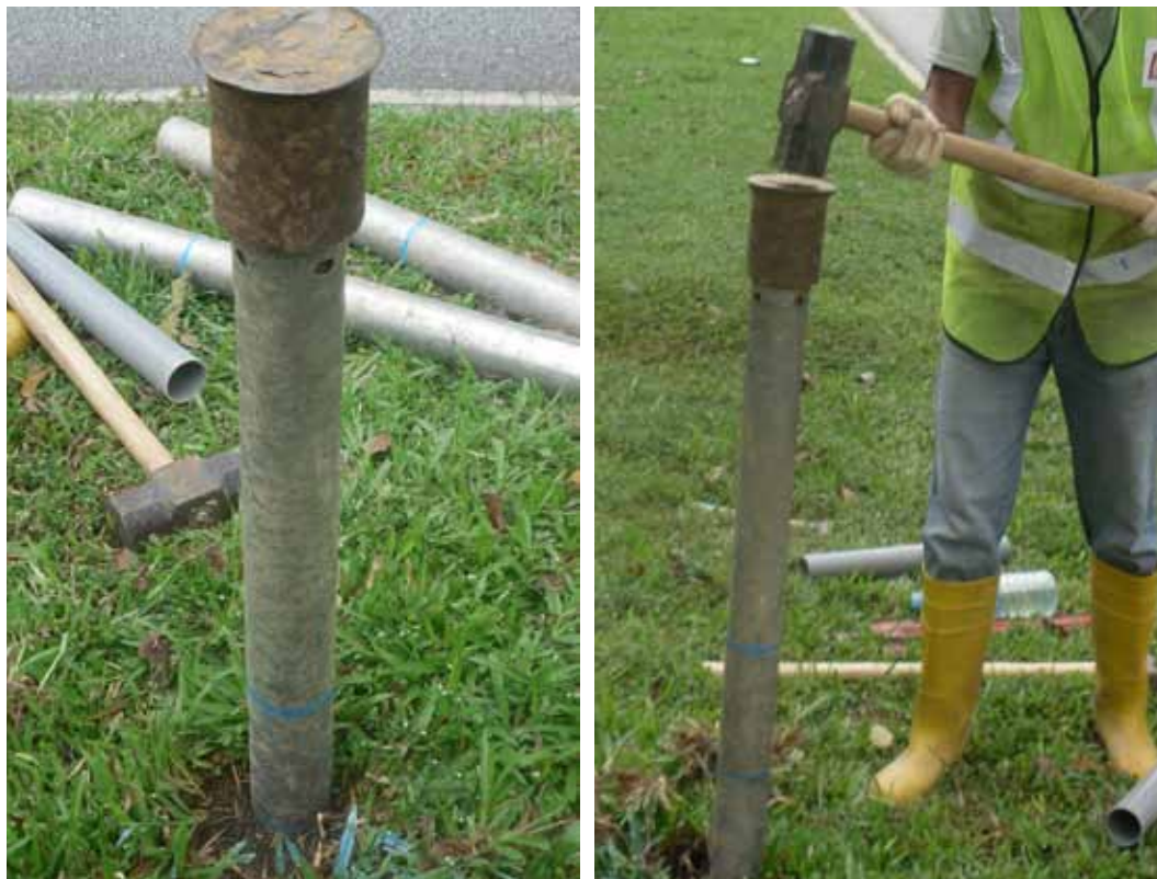
Fig 4. Collection of in-depth undisturbed soil samples.
