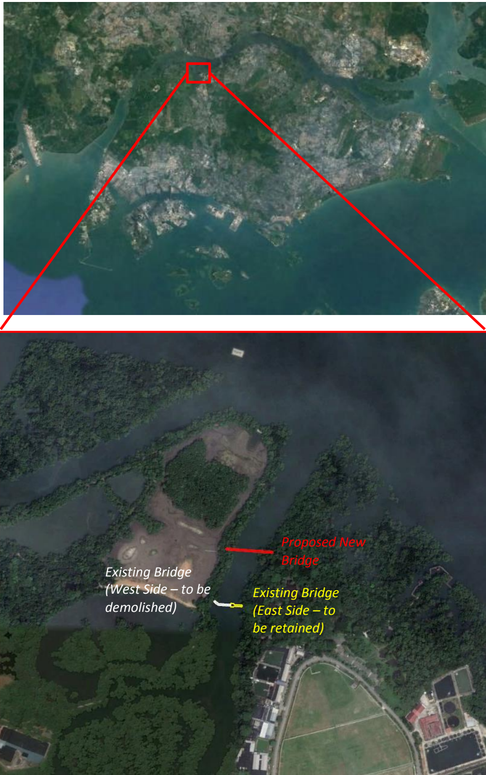
Figure 1-1: Location and outline of the existing and proposed main bridges across Sg Buloh Besar
