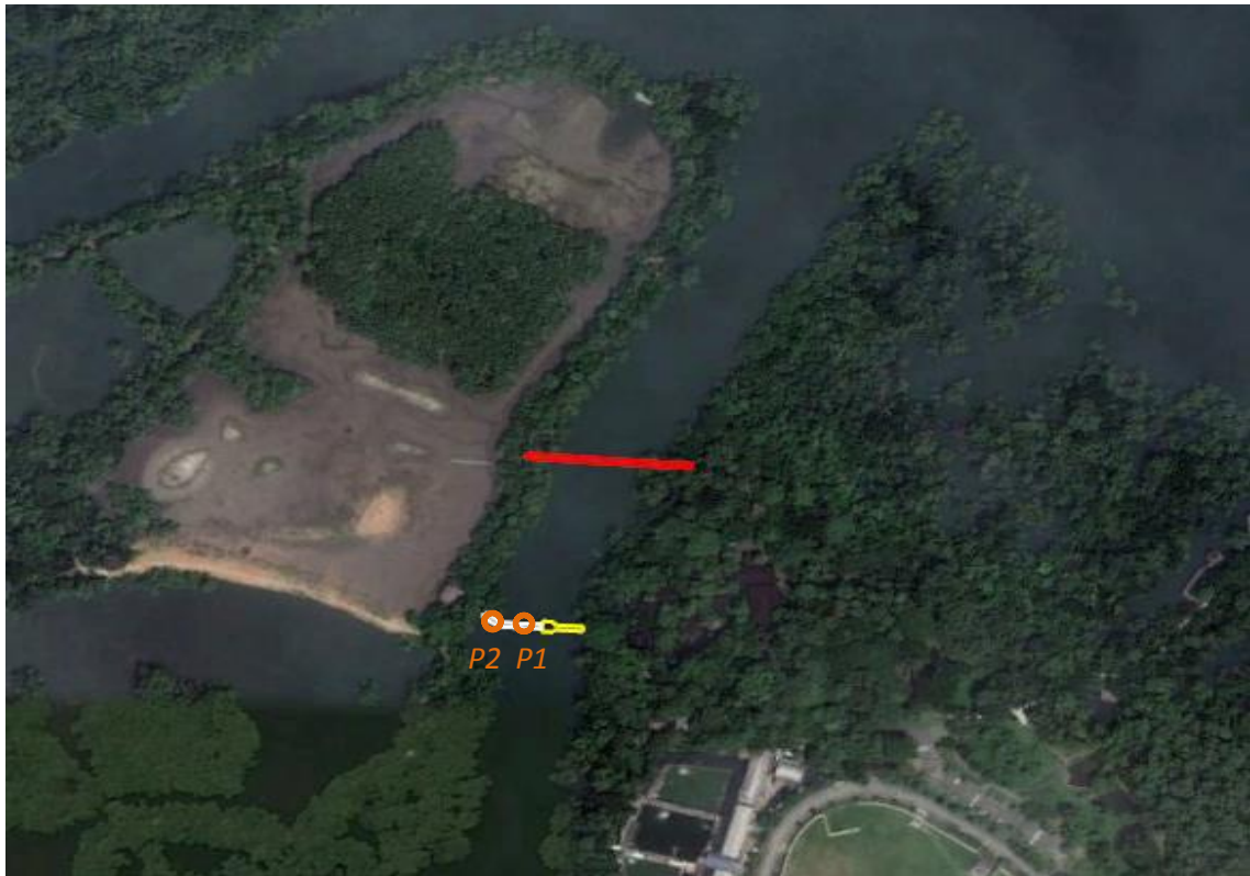
Figure 6-1: Selected discharge points of sediment plume for numerical modelling: P1 – at the river centre, P2 – close to the west bank.
