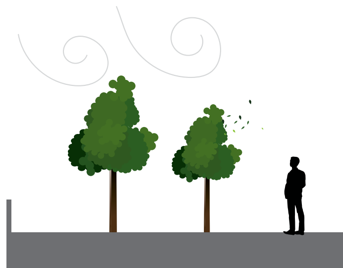
Porous canopy allow wind to pass through, thus reducing wind loads and impacts.
