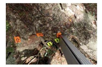
Resistograph drilling (R1) taken at trunk to root junction shows decay after 21cm. This indicates that decay has already infected partially at the underside of the tension root (BR1).
