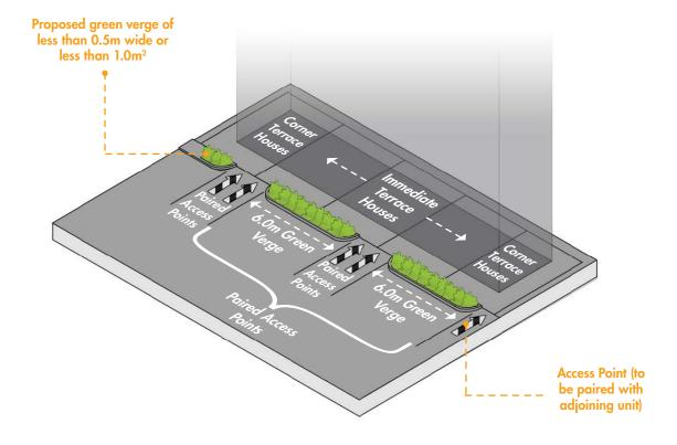
d. In upgrading projects where the existing open drains are converted into box culvert (i.e. footpath cum drain), the existing footpath should be converted into green verge. Refer to the following illustration.
