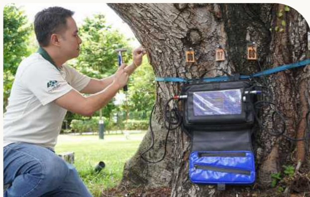
Remote Tree Management System (RTMS) and Internet-of-Things (IoT) sensors are some digital tools that will be integrated into Maven 2, a centralised platform for greenery management to enhance tree inspections and monitor park amenities.
