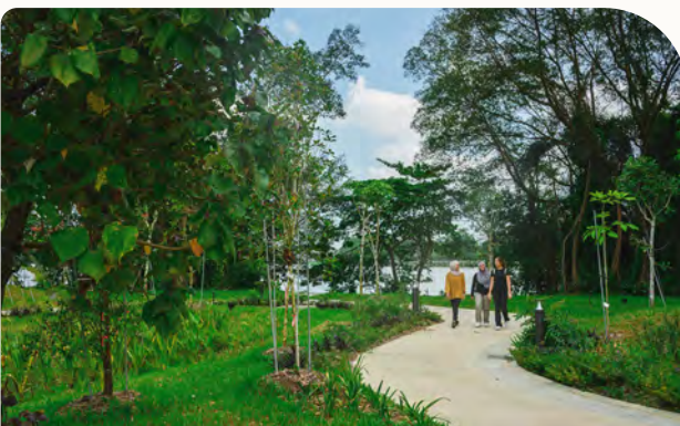
Footpaths in the northern section of Jurong Lake Gardens are constructed from carbon dioxide mineralised concrete and act like a carbon sink. During the production of this concrete, industrial waste carbon dioxide is permanently embedded into it.
