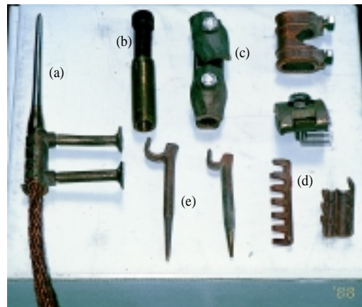
Some of the materials used for the lightning protection system. Clockwise from left: copper conductor cable attached to an air terminal (a), part of the ground rod, (b), two types of ground connectors (c), three types of cable fittings (d), and two different size of tree drive fasteners (e).
