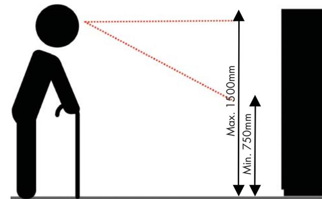
An example of a directional marker with suggested clearance perimeter for the information displayed
