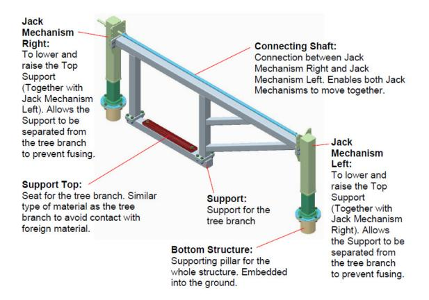
The dynamic support system strives to provide an environment for the iconic Tembusu Tree's lateral limb to sway naturally under wind while supporting it at the same time. It aims to facilitate the strengthening of the tree branch and eventually enable the branch to support itself without any external supports.
